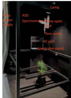
Figure 1: Setup used by William Cornforth as part of his PhD collection program to collect spectra collected from inoculated and control seedlings.
